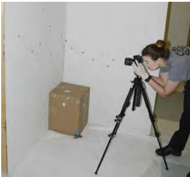
Figure 1: Photographs of the bloodstains were captured with black and white targets for image alignment.
