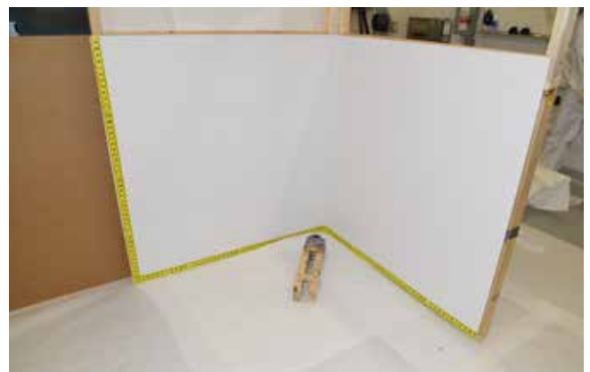
Figure 5: The setup with the striking surface that created the two sided pattern on two perpendicular walls for the reproducibility evaluation.
