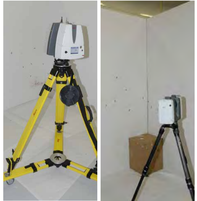
Figure 2: The setup was scanned using the Leica ScanStation P40 and Leica RTC360.
