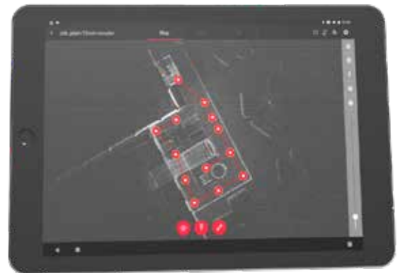
Auto-aligned point clouds in 2D view mode
