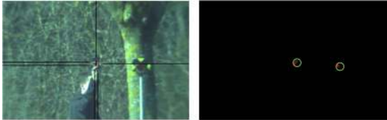
Figure 4 - Left: test setup with two prisms (360° prism GRZ122 and round prism GPR121) in the field of view of the instrument. Right: visualisation of the two spots as ATRplus sees them.
