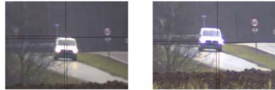
Figure 3 - ATRplus (left) is correctly locked onto the prism on the top of the car. ATR (right) tries to lock onto the car headlights.
