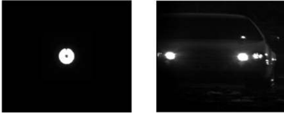
Figure 2 - Images from the CMOS sensor. Left: prism spot. Right: two car headlights and sun reflections on the car.
