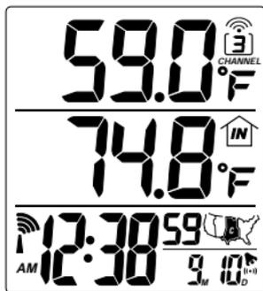
If no signals are received, blanks "----" will be displayed and the kinetic wave icon will show "
