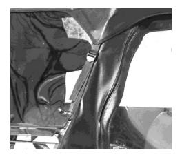
12. Next take the other two long straps and wrap them around the roll cage in the rear just under door and rear window at the very bottom of the roll cage. Pull the strap up and connect to the buckle at the rear of the top.
