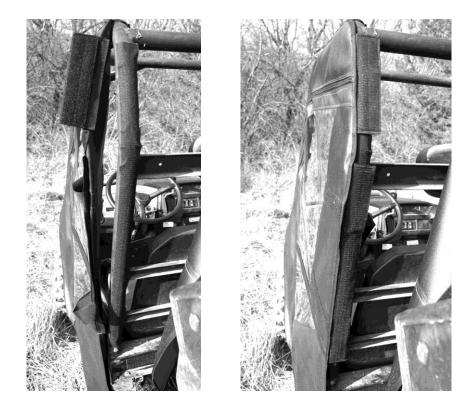
5. Once all the Velcro is in place the last thing to do is install the screw snap studs. NOTE: The best way to install the snap studs is to put them in the sockets in the door first. Then push them into the plastic to make a mark. Then pull the screw stud out and screw it into the plastic where the mark was made. See Photos Below.
