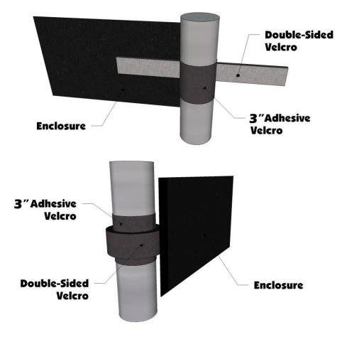
4. Next take the 38" adhesive Velcro strips and run it down the back of the roll cage facing towards the rear of the vehicle. Start at the bottom and work your way up the bar. You will see the double-sided Velcro tabs sewn along the back of the doors. See photos below.
