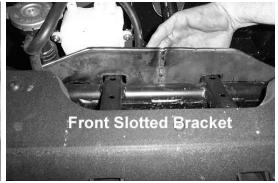
5. Place spacer between the shock mount tabs and insert the 10mm x 65mm hex bolt through the slotted bracket and spacer.
