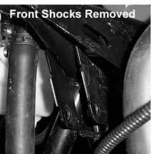
4. Insert the front slotted bracket on the backside of the front cross member. NOTE: We have removed the front plastic so you can see how this bracket is installed. This is
