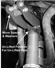
5. Once you have repositioned the shocks, torque all the nuts and bolts tight, you can then lower the jack.
