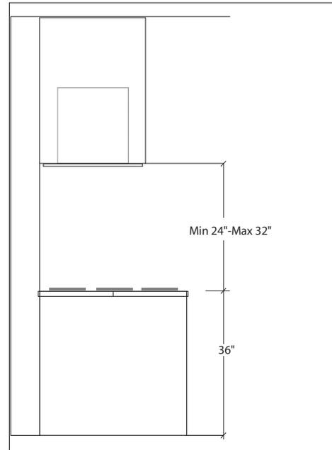
Minimum mount height between range top to hood bottom should be no less than 24".
