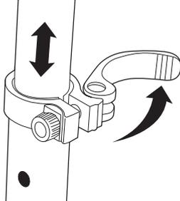
**5** To adjust the height of the handlebars, unlock the extension tube by pulling outward on the quick-release lever and pushing the button located on the extension tube. Slide the T-tube to the desired position and secure by pushing inward on the quick release lever.
