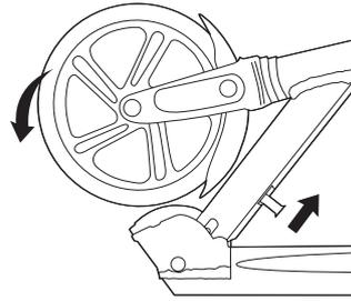
**3** To release the folding mechanism, hold the T-tube with one hand between the collar clamp and the quick-release lever and place your foot on the deck plate. With the other hand, pull the joint lever up to release the steering column from the locked position and allow you to pivot it to the upright position.
