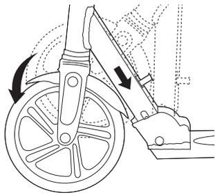
**4** The Joint lever is spring-loaded and will automatically lock in the upright position when fully upright.
