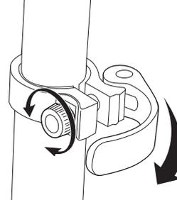
**6** The tension of the quick-release lever can be adjusted by tightening or loosening the allen bolt. Be careful not to over-tighten. You should always be able to open and close the quick-release lever by hand and the T-tube should slide freely with the quick-release open.
