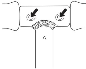
**2** Make certain the spring-loaded button engages the hole in the T-bar for each handlebar.
