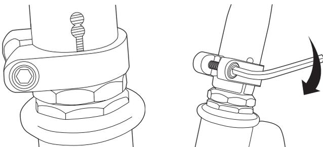
Using the 5mm Allen wrench, check that the collar clamp bolt is tightened securely. This item is tightened and quality inspected at the factory, but there is a slight chance that the effects of shipping or handling may have caused this bolt to loosen.
