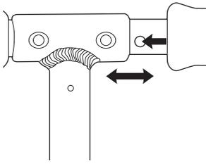
**1** Insert and secure the left and right handlebars by pressing the spring-loaded buttons and inserting them into the T-tube.
