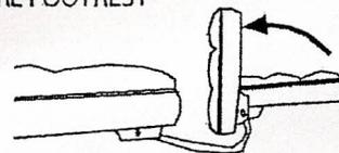
1. Grasp the Footrest in the center and pull forward to a vertical position.
