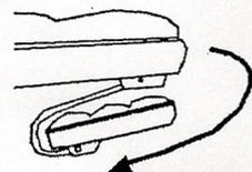
2. Push the Footrest down and backward until it is completely under the seat.
