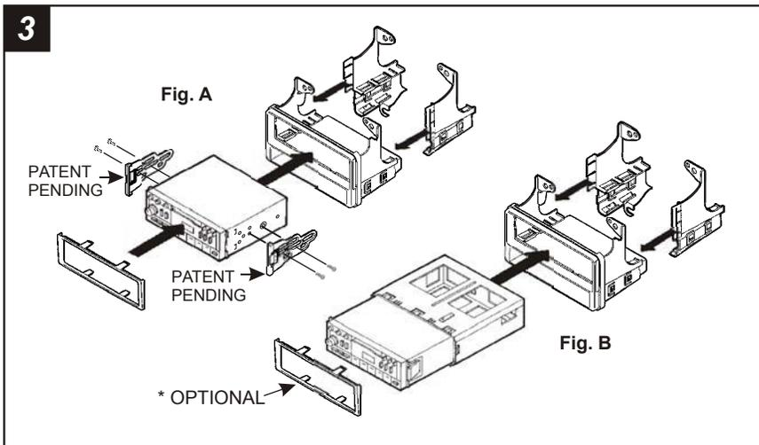
**ISO HEAD UNITS:** Slide the Mounting Brackets onto the sides of the Radio Housing until the side clips engage. Mount the ISO Brackets to the head unit with the screws supplied with the unit. Slide the head unit into the radio opening until the side clips engage. Snap the Trimplate into the Radio Housing. (see Fig. A).
