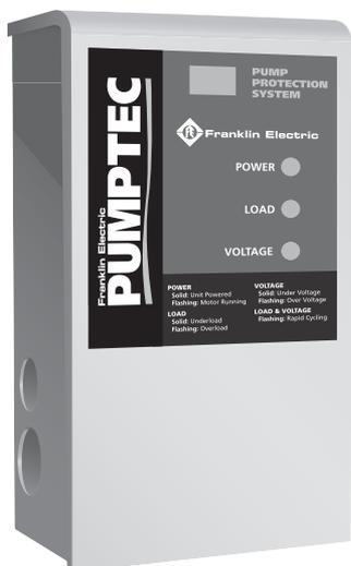
Pumptec is a microcomputer based pump protection device that continuously monitors motor load and power line conditions to provide protection against dry well conditions, waterlogged tanks, and abnormal line voltage conditions.
