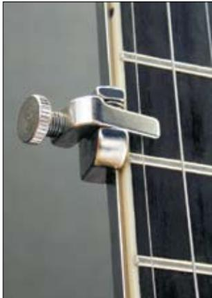
It operates on a lever principle, not a spring, thereby providing enough pressure to hold the string solidly in place without muting the tone. It slides on a slim, dovetailed bar which mounts flush to the neck, making it sturdy and unobtrusive. The compact bar requires only two mounting screws and occupies less space on the neck than our earlier version. The old style with longer bar (greater range, 3-point mount) is still available as a special order.
