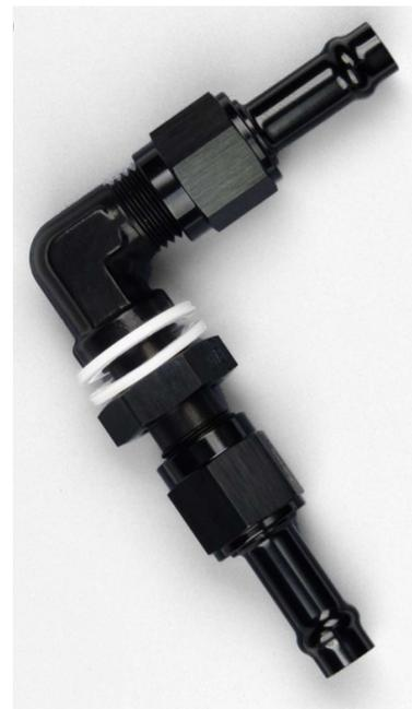
Instead, use the OE feed line for the return. But what to do about a feed line? We offer a 3/8-inch fuel port fitting (shown.) It requires that a hole be drilled in the top of the tank, only in the cover plate through which the fuel pump will be accessed, and only after the cover has been removed and thoroughly washed and dried. WE DO NOT RECOMMEND DRILLING YOUR FUEL TANK, ONLY THE COVER PLATE.
