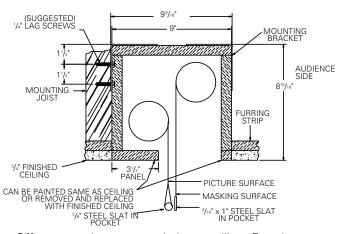
Offset mounting, recessed above ceiling. For plaster, dry wall, tile or paneling. Bottom of case painted same finish as ceiling.
