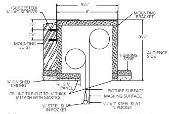
Offset mounting, recessed above ceiling. May be adapted for  $^3/_4$ " ceiling, but cut to  $^1/_4$ " thick under screen case and panel.
