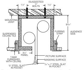
Flush mounting, recessed above ceiling. For use with dropped ceiling. May also be adapted for use with acoustical or other ceiling 3/4" thick but cut to 1/4" thick under screen case and panel.
