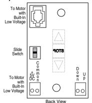
Please Note: 5V DC must be connected to be able to set limits using the wall switch.
