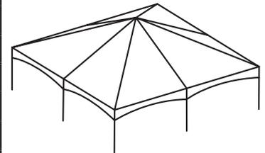
1. The layout begins with the frame parts being laid out on the ground in the approximate location that they will be when the frame is assembled. The perimeter parts are laid out to form the perimeter, and the roof support parts are placed in the interior in their general locations. Laying out the parts in this way facilitates the assembly. (See Diagram)
