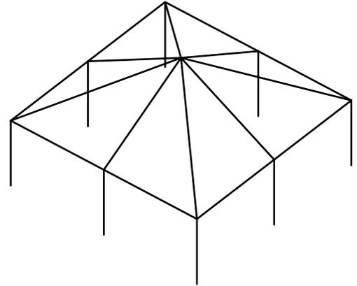
1. The layout begins with the frame parts being laid out on the ground in the approximate location that they will be when the frame is assembled. The perimeter parts are laid out to form the perimeter, and the roof support parts are placed in the interior in their general locations. Laying out the parts in this way facilitates the assembly. (See Diagram)
