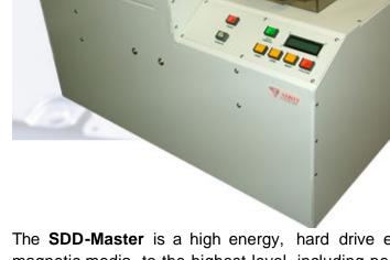
The **SDD-Master** is a high energy, hard drive eraser designed to offer complete and secure erasure of magnetic media, to the highest level, including perpendicular recording hard drives. The SDD-Master is also capable of erasing data storage media including DLT, LTO, 8mm, DDS and more.
