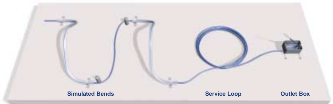
Installation Stress Test Set-Up
