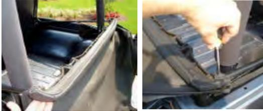
**Step (7) :** Flip the top fabric back over into the rear of the vehicle (so that the fabric lays backing side up) to expose the plastic strip along the edge of the fabric. Remove the eight or fourteen screws that secure the fabric to the header, setting the screws aside for use in the installing the new top. Then remove the old top fabric from the vehicle.
