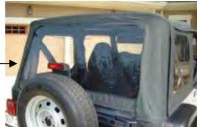
Make sure that the tailgate is centered and is securely in the mounts. Then tuck the flaps on the rear window under the top fabric.
