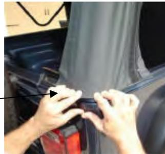
**Step (6) :** Close the header latches to secure the front of the top to the windshield. Catch the hook in the slot in the windshield frame and then close the lever over it so that it lays flat against the windshield frame.
