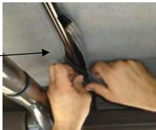
**Step (8) :** Locate the left and right quarter window panels and orient them with the zipper slider about 10" - 12" along the top.
