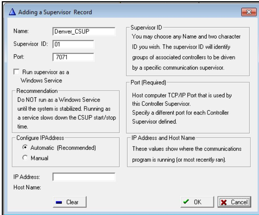
Enter a unique name of the CSUP that will manage your doors. This name will be used to reference the Controller Supervisor within the application.
