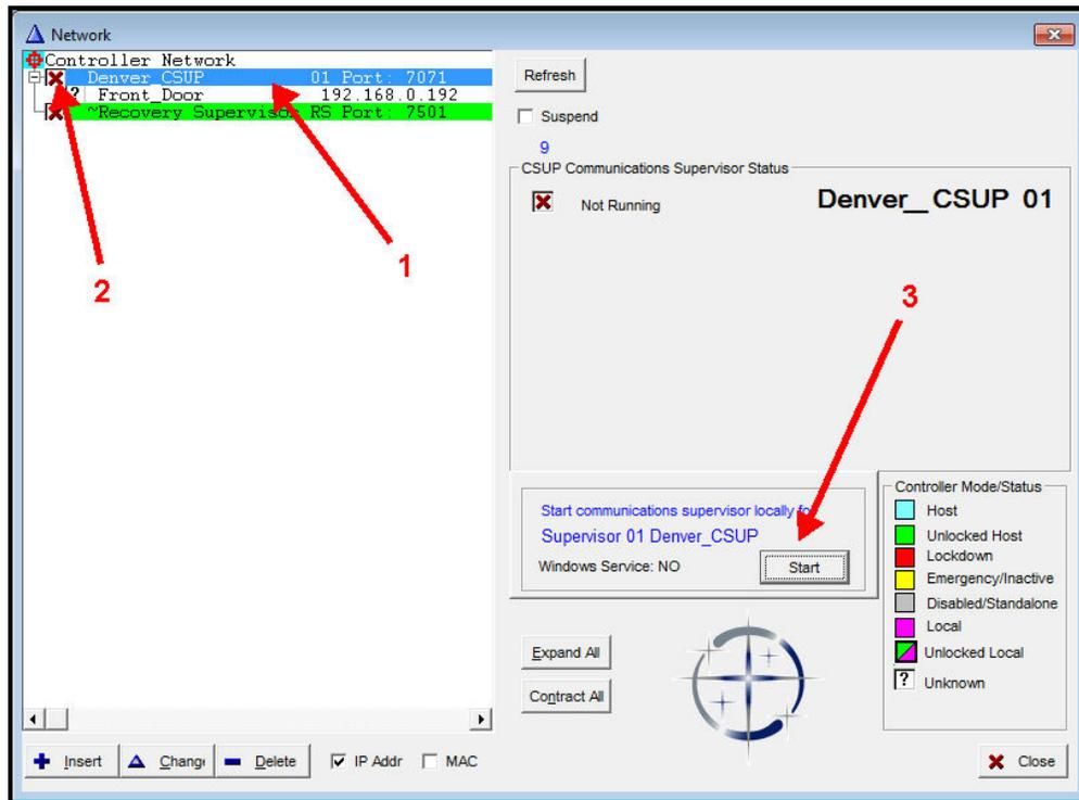
Note the CSUP’s status is shown with a red “X” (Arrow #2). When the CSUP is selected, the window will display a “Start” button for that CSUP (Arrow #3). Clicking this button will start communication to each of the doors listed for that CSUP.
