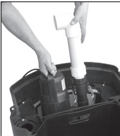
Place the pump and discharge plumbing assembly into the SAVIO Skimmerfilter™.
