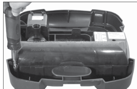
9. Replace uv cover and secure with screws.
