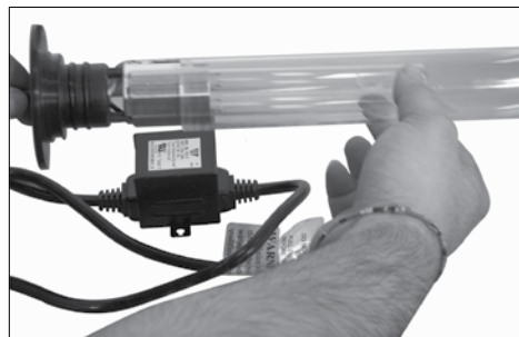
7. Carefully slide quartz sleeve over bulb and onto ballast making sure sleeve is pushed all the way over both "O" rings and next to the flat end of the ballast assembly.
