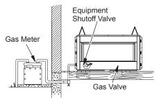
Figure 15 - Checking Gas Joints for Natural Gas Fireplace
