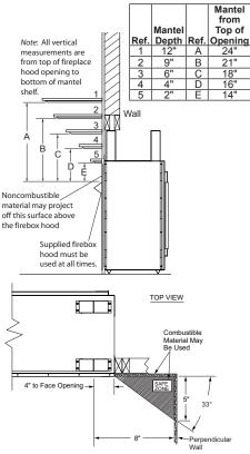
Figure 7 - Clearances for Combustible Mantels
