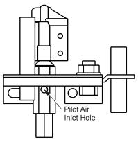
Figure 40 - Pilot Inlet Air Hole
