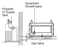
Figure 14 - Checking Gas Joints for Propane/LP Gas Fireplace
