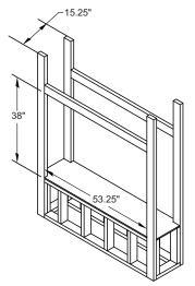
Figure 5 - Framing Clearances for See-Thru Application
