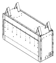
Figure 18 - Removing Rear Panel for See-Thru Applications
