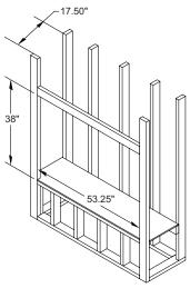
Figure 4 - Framing Clearances for One Sided Application
