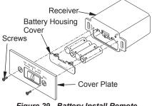
Figure 29 - Battery Install Remote Control Receiver
