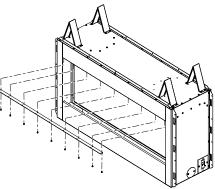
Figure 19 - Removing for See-Thru Applications
