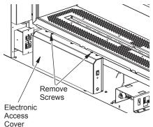
Figure 27 - Removing Control Access Cover (Face Bottom not shown for Clarity)
