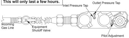
Figure 30 - Turning Equipment Shutoff Valve to the OFF Position
