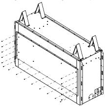
Figure 16 - Installing Rear Panel for Regular Applications
