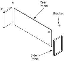
Figure 21 - Removing Rear Interior Wall for See-Thru Applications
