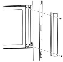
Figure 23 - Installing Side Face Filler for See-Thru Applications
