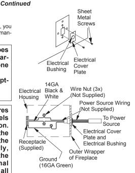
Figure 9 - Connecting Electricity
