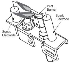
Figure 41 - Correct Pilot Flame Pattern
