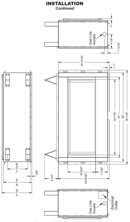
Figure 8 - (V)LVF43 Series Dimensions
