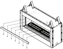
Figure 17 - Installing Hood
