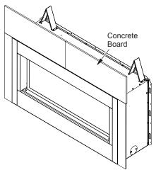
Figure 6 - Installing Concrete Board
