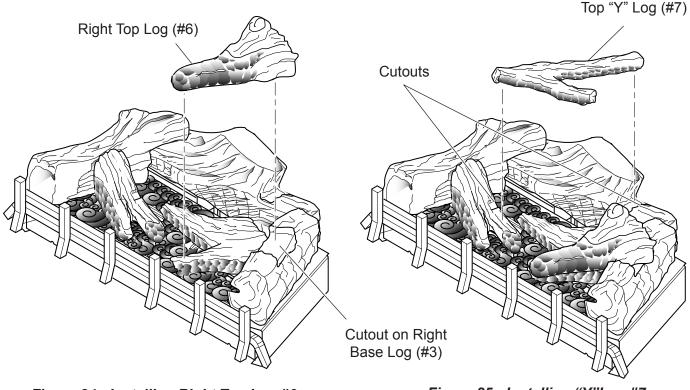
Figure 24 - Installing Right Top Log #6
