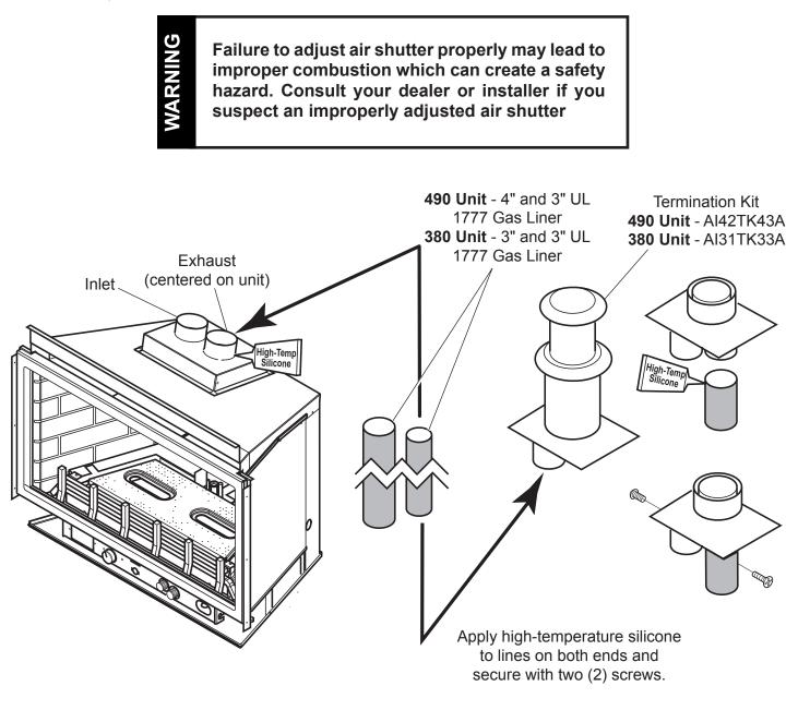
Figure 7 - Connecting Exhaust Pipe to Heater
