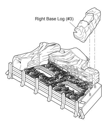
Figure 21 - Installing Right Log #3
