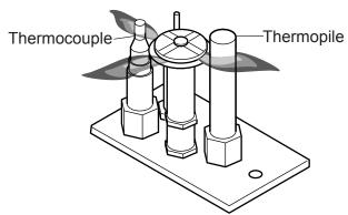
Figure 42 - Typical Pilot Flame
