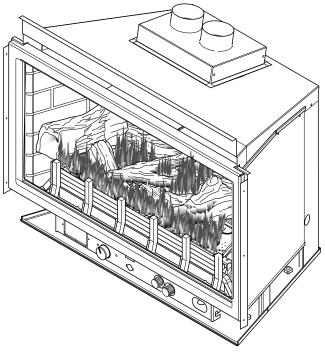
Figure 41 - Typical Burner Flame
