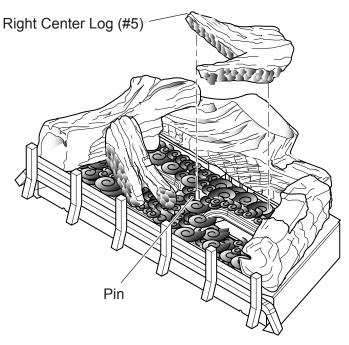
Figure 23 - Installing Right Center Log #5
