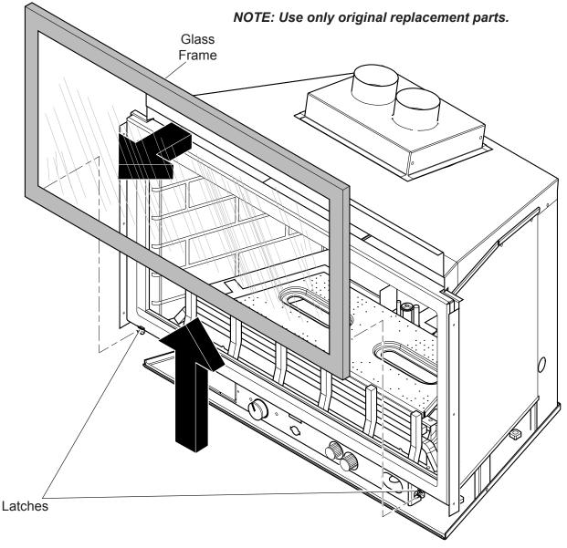
Figure 40 - Removing Door
