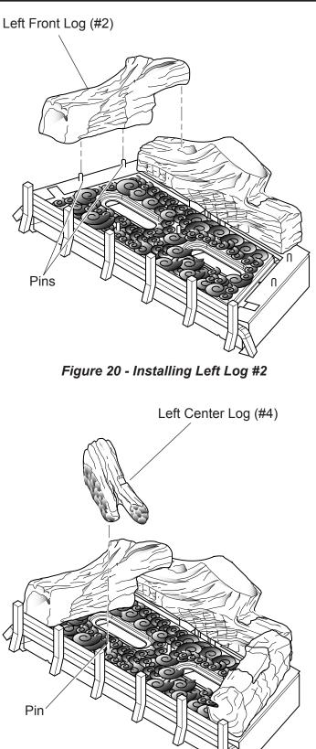
Figure 22 - Installing Left Center Log #4
