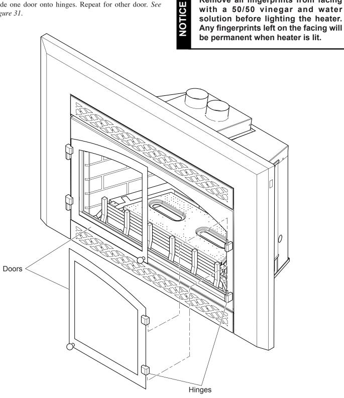
Figure 31 - Installing Doors
