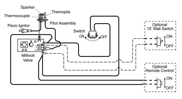
Figure 17 - Wiring Diagram for Wall Switch
