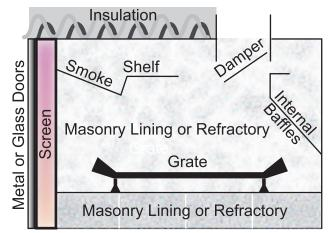
Figure 5 - Metal Fireplace Zero-Clearance Requirements
