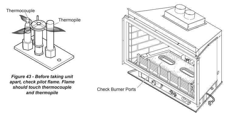
Figure 44 - Checking Burner Ports and Burners
