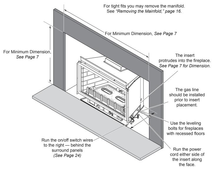
Figure 4 - Insert Placement
