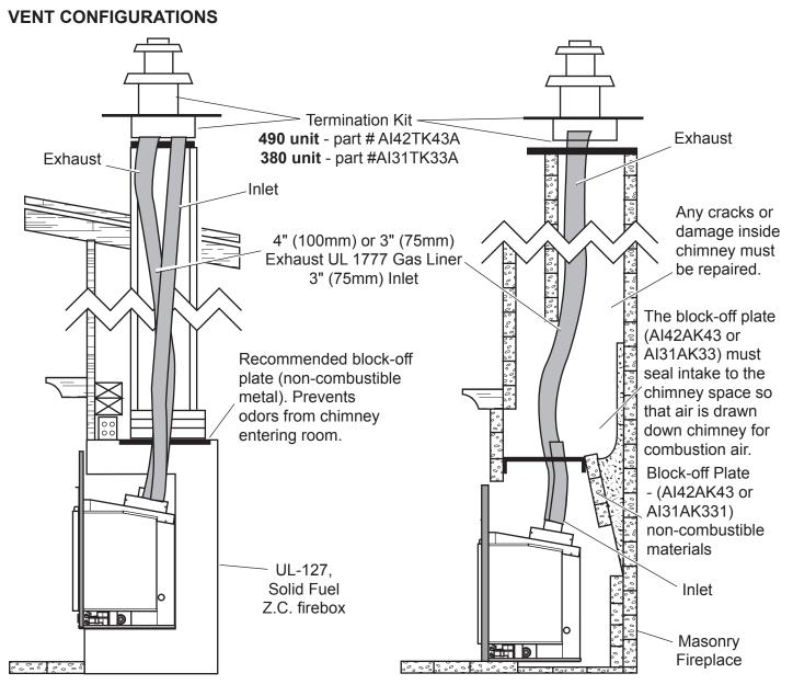
Figure 8 - Inlet and Exhaust Reline
