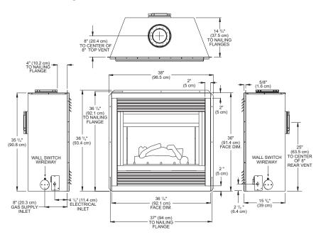
Figure 9 - Rear/Top Common Dimensions
