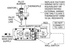
Figure 42 - Millivolt Ignition Wiring Diagram
