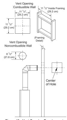
Figure 12 - Vent Opening Requirements
