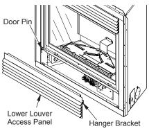
Figure 56 - Removing Lower Louver Access Panel
