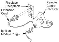
Figure 48 - Connecting WRC Remote Control Electronic
