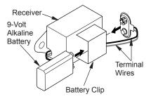
Figure 45 - Attaching Alkaline Battery to Receiver
