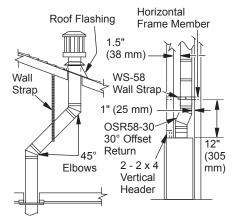
Figure 26 - 45° and 30° Offset with Wall Strap
