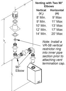
Note: Vertical (V<sub>1</sub>) + Vertical (V<sub>2</sub>) = 40' Max. Max. Horizontal Above 14' Vertical = 20'
