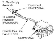
Figure 52 - Connecting Flexible Gas Line to Millivolt Valve
