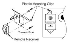
Figure 46 - Mounting Remote Receiver to Bracket
