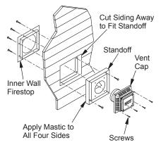
Figure 14 - Installing Siding Standoff (Combustible Exterior Wall)
