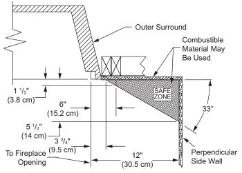
Figure 8 - Side Clearances for Combustible Materials
