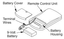
Figure 47 - Installing Battery in Hand-Held Remote Control Unit
