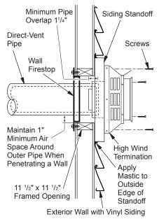
Figure 17 - Typical Horizontal Termination Cap Mounting with Additional Siding Standoff Installed
