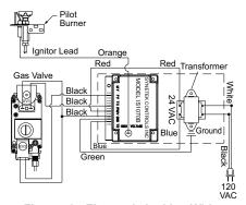
Figure 43 - Electronic Ignition Wiring Diagram
