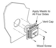
Figure 13 - Installing Horizontal Vent Cap
