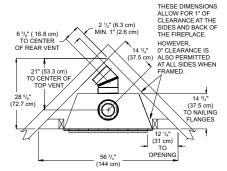
Figure 6 - Framing Clearances for Corner Installation
