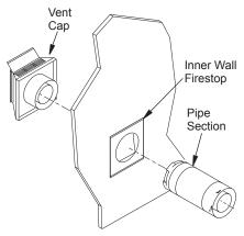
Figure 16 - Installing Inner Wall Firestop
