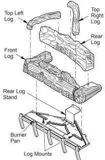
Figure 59 - Installing Logs
