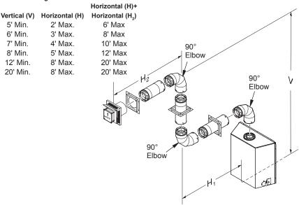
Figure 25 - Horizontal Termination Configuration for Venting Using Three 90° Elbows (Model (V)CD36T)
