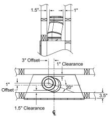
Figure 27 - OSR58-30 Offset and Return for (V)CD36T Series Units
