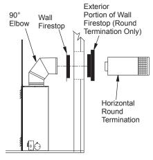
Figure 20 - Horizontal Termination **Configuration Round Termination** (Model (V)CD36T)
