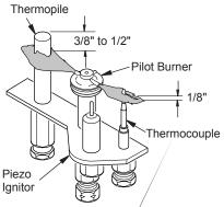
Figure 68 - Pilot Assembly (Millivolt)
