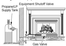
Figure 54 - Checking Gas Joints for Propane/LP Gas Fireplace
