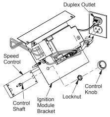
Figure 38 - Attaching Speed Control to Firebox (Electronic Models)
