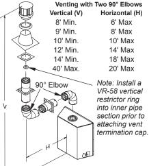
Figure 32 - Vertical Venting Configuration Using Two 90° Elbows (Model (V)CD36T with Vertical Round High Wind Termination)
