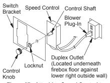
Figure 37 - Attaching Speed Control to Firebox (Millivolt Models)
