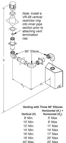
Figure 31 - Vertical Venting Configuration using Three 90° Elbows (Model (V)CD36T with Vertical Round High Wind Termination)
