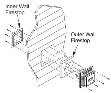
Figure 15 - Installing Outer Wall Firestop (Combustible Exterior Wall)
