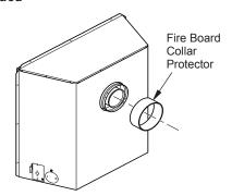
Figure 4 - Removing Collar Protector (Rear Vent Fireplace)
