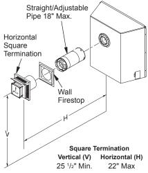
Figure 18 - Horizontal Termination Configureation for Flush Installation (Model (V)CD36R)
