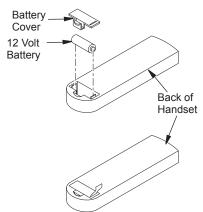
Figure 49 - Installing Battery Into Handset WRC
