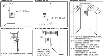
Figure 10 - Minimum Clearances for Termination Cap
