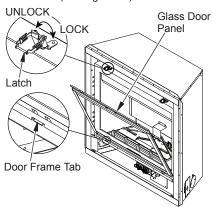
Figure 58 - Removing/Replacing Glass Door
