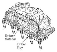
Figure 60 - Applying Ember Material
