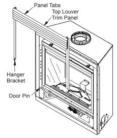
Figure 57 - Removing Top Louver Trim Panel
