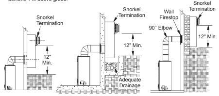
Figure 23 - Snorkel Termination Configuration For Below Ground Installation
