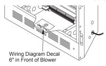
Figure 39 - Location of Wiring Diagram Decal (Model May Vary From Illustration)
