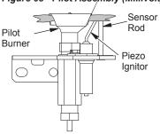
Figure 69 - Pilot Assembly (Electronic)
