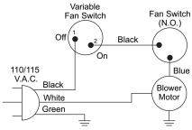
Figure 41 - Blower Wiring Diagram for Thermostat-Controlled Models
