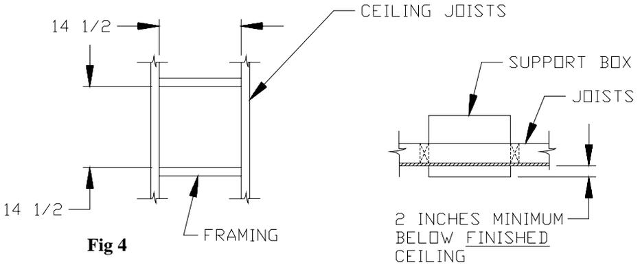
for specific framing and clearance dimensions. Mark appropriate cutting lines around the center point. Cut a square hole in the ceiling for a **Square Support Box**, or a round hole for a **Round Support Box**. Frame a level, square opening centered over the hole which you have cut. (Figures 3 and 4).
