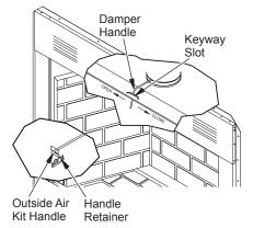
Figure 22 - Damper and Air Kit Handle
