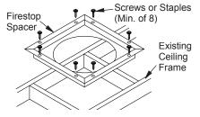
Figure 11 - Firestop Spacer with Attic Space Above Ceiling
