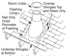
Figure 13 - Flashing Installation
