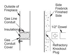
Figure 19 - Gas Line Knockout
