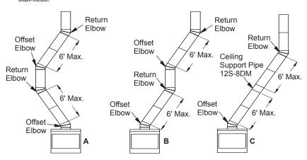
Figure 7 - Typical Offset Terminations
