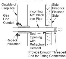
Figure 20 - Gas Line Installation
