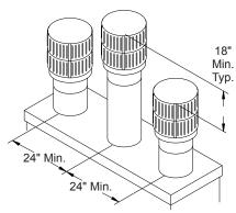
Figure 16 - Multiple Chase Installation
