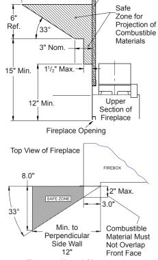
Figure 4 - Mantel Clearances to Combustible Material
