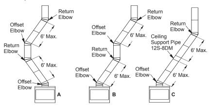
Figure 7 - Typical Offset Terminations
