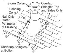
Figure 13 - Flashing Installation
