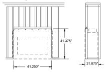
Figure 1 - Framing Dimensions
