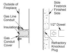
Figure 19 - Gas Line Knockout
