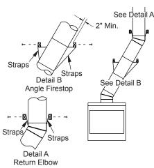
Figure 8 - Ceiling Support Pipe 12S-8DM
