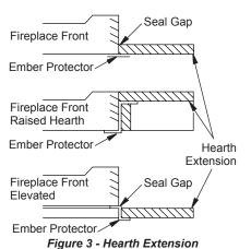
WARNING: Hearth extension is to be installed only as shown in Figure 3.
