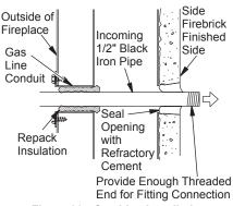
Figure 20 - Gas Line Installation
