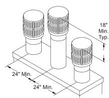
Figure 16 - Multiple Chase Installation
