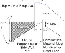
Figure 4 - Mantel Clearances to Combustible Material
