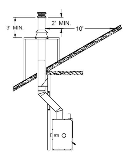
Figure 24 – Example of a combustible chase enclosure installation above the roof
