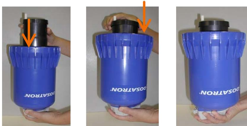
Insert the piston into the upside down bell housing half way down. Then let go of the piston. The piston should be snug in the upper housing and should not fall in. If it does, the piston shell needs to be replaced. Also inspect the inside of the bell housing and look for deep vertical scratches or excessive wear. If this is the case, the bell housing needs to be replaced.
