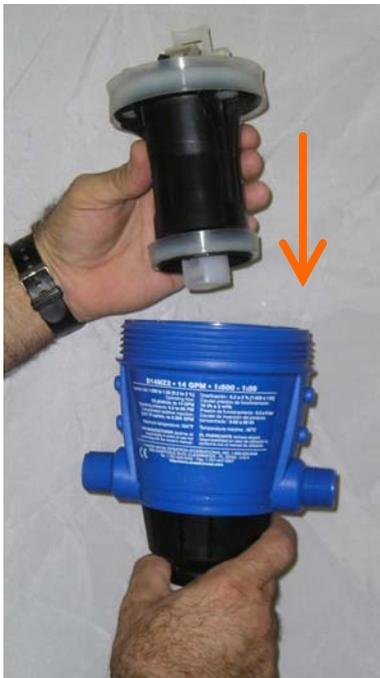
Insert the lower part of the piston halfway down the body. Holding onto the top of the piston, let go of the body. The piston should be snug in the body, and the body should not fall off, if it does the lower piston shell needs to be replaced.
