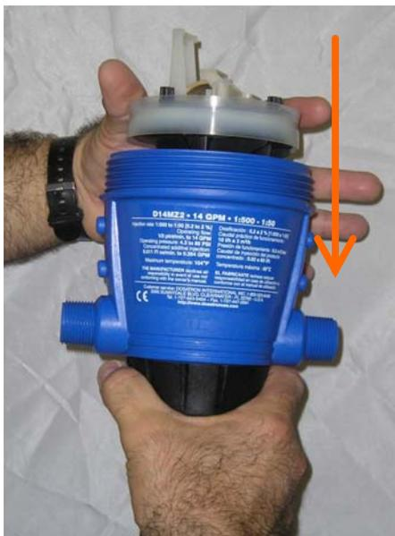
To reset the piston, remove the bell housing and the piston. Press down on the push rod until it clicks (it may not click if the piston was traveling up when the unit stopped). Then push the piston into the lower housing until it clicks. Replace the upper bell housing and screw on.
