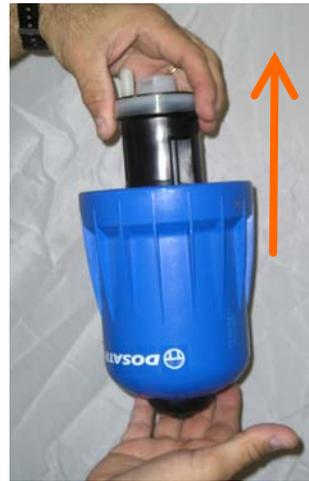
Insert upper portion of piston into the bell housing halfway down, turn the bell housing upside down. Holding the bottom of the piston, let go of the bell. The piston should be snug in the bell housing and the bell housing should not fall off. If it does, the upper piston flange needs to be replaced.
