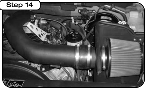
Your installation is now complete. Check after a few hours of operation all hoses and clamps are tight and that all electrical components are secure. Close hood slowly to verify hood clearance.
