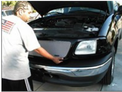
Picture #17: Install the grille shell.
