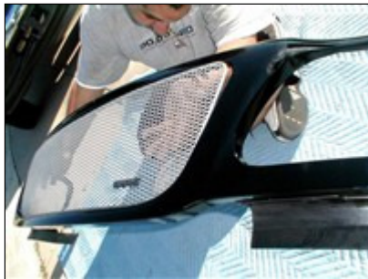
Picture #14: Install the GrillCraft Grille from the front side of the shell opening.
