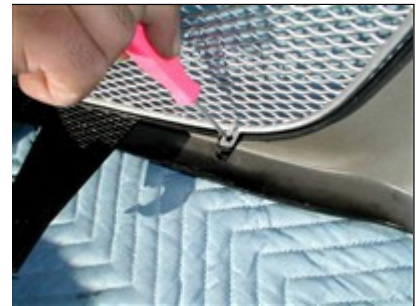
Picture #15: While holding grille in place mark the mounting bracket center hole using a sharp scribe.
