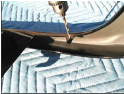
Picture #16: Drill a 3/16 hole for the mounting screws and fasten grille with supplied screws and clips.
