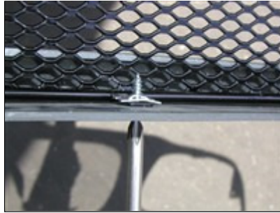
Picture #17: Fasten the bottom section of the grille first.
