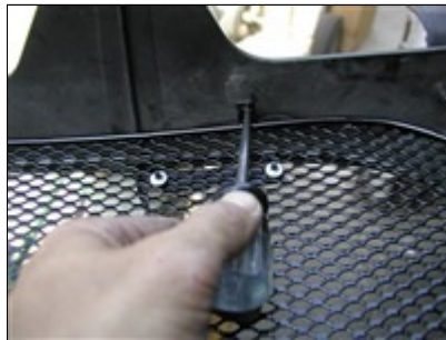
Picture #14: Insert the mesh grille from the backside and mark the center of the mounting brackets.
