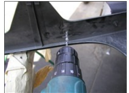
Picture #15: Using a 3/16 drill bit drill for the mounting screws.
