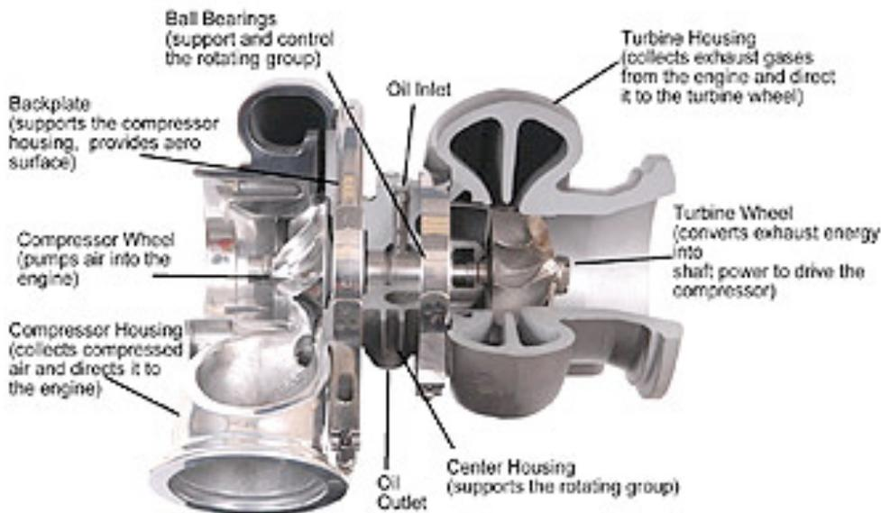
The ball bearing cartridge design is a single sleeve system that contains a set of angular contact ball bearings on either end, whereas the traditional bearing system contains a set of journal bearings and a thrust bearing.
