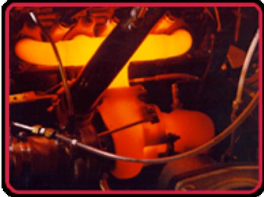
To minimize the effects of heat soak-back, AVO only uses water-cooled turbo center housings. These use coolant from the engine to act as a heat sink after engine shutdown, preventing the oil from coking. The water lines utilize a thermal siphon effect to reduce the peak heat soak-back temperatures after you turn the car off. Please take care with the layout of the pipes, which should minimize peaks and troughs with the (cool) water inlet on the low side.
