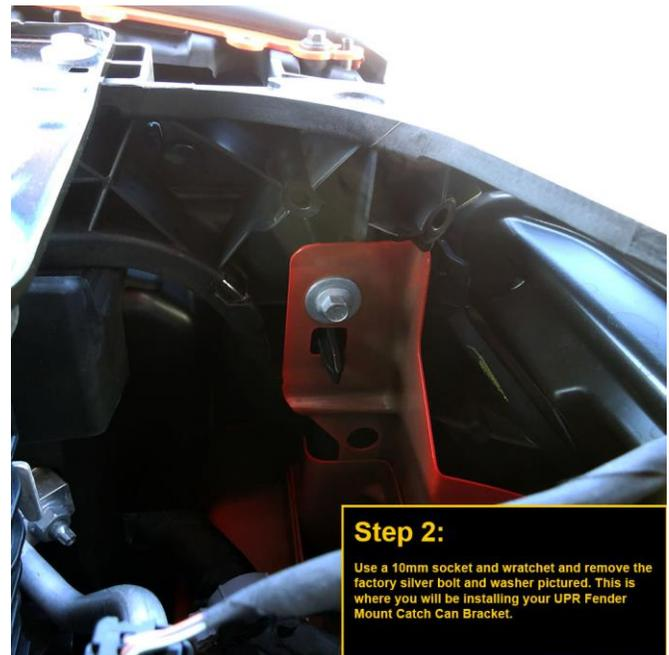
Use a 10mm socket and ratchet to remove the factory silver bolt and washer pictured. This is where you will be installing your UPR fender mount catch can bracket.
