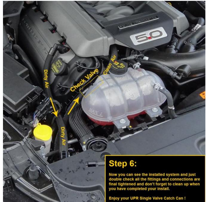
Now you can see the installed system and just double check all the fittings and connections are final tightened, reinstall the radiator cover and don't forget to clean up when you are completed your install.
