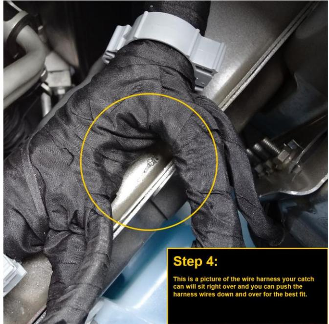
This is a picture of the wire harness your catch can will sit right over and you can push the harness wires down and over for the best fit.
