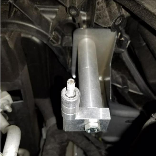
Use a socket and ratchet to snug your UPR fender mount bracket with the supplied spacers in place.
