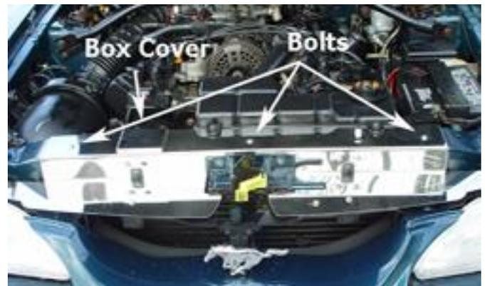
4). Remove the bolt from the center of the core support. 5). Remove the four bolts holding the two airbag sensors to the core support. 6). On 94-96's replace the factory radiator support bracket on the passenger side with the new bracket. On 97-98's replace both factory radiator support brackets with the ones provided.
