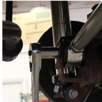
8. Unbolt the pan hard bar bolt but do not remove it just back it out till the factory nut comes off but you can leave the bolt in to keep the bar in place.
