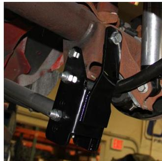
12. Install the Passenger side bracket. The 12mm bolt goes into the top bolt hole or reinstall the factory axle weight. Put the 14mm x110 bolt with spacer through the second hole. The back strap is secured with 1/2 bolt, washer and nut. The control arm bolts in with 14mmx110 bolt.
