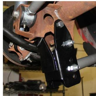
13. Tighten all the driver and passenger side hardware.
