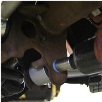
7. Remove the lower control arm bolts on the axle side and let the control arm hang from the body side.
