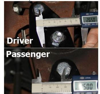
14. If your car does not have the axle weights or holes already there you will have to drill the top 12mm locating hole. The driver side hole should be 2.650" from the front of the axle bracket. The passenger side should be 1.50" from the front of the axle bracket.
