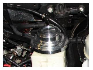
I placed a bead of silicone adhesive along the inside edge of the cover and let it dry set completely. Next, I simply pushed the cover onto the cap. The silicone provides enough resistance to hold the cover firmly in place on the cap while still allowing me the ability to pull it off the cap whenever I need to access steering fluid (and that's not very often!)
