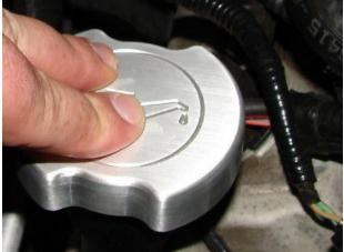
For the oil filler cap, place a small amount of clear automotive silicon adhesive on the underside of the billet cover. Once you've cleaned and dried the oil filler cap place it back on the oil filler tube and then place the billet cover on top of this. Hold it down firmly for a couple of minutes until it starts to set.
