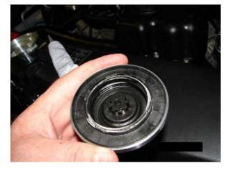
Next, the brake fluid and coolant cap covers. The UPR pieces press fit onto these but I added a small amount of clear silicone adhesive on these as well.
