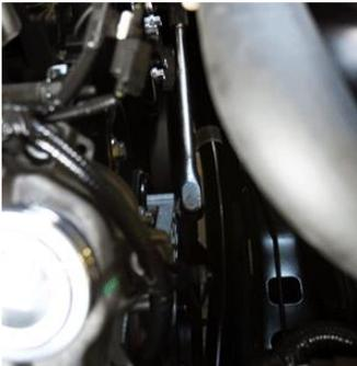
Using a socket wrench or breaker bar release the tension on the stock tensioner and remove the belt from the alternator pulley so it has enough slack.
