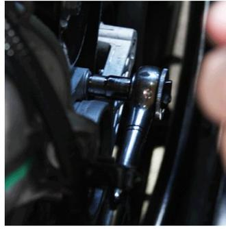
Using a 10mm socket remove the three bolts holding the stock tensioner to the timing cover.
