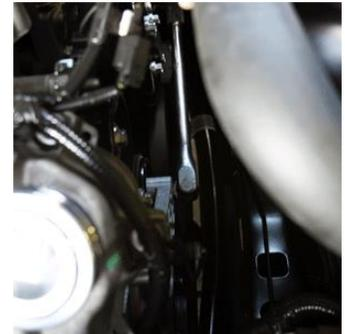
Make sure the belt is still properly routed and using a breaker bar or socket wrench compress the tensioner and reconnect the belt on the alternator pulley.
