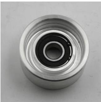
**03/04 COBRA Owners:** When using this tensioner on the accessory drive you have to flip the billet pulley backwards and put each of the three spacers behind the tensioner mount. The picture above shows the back of the pulley that normally faces the timing cover. It should be facing forward for the 03-04 Cobra so it clears the timing cover. If using the tensioner for the supercharger drive you have to reuse your stock ribbed tensioner pulley that came on your car.
