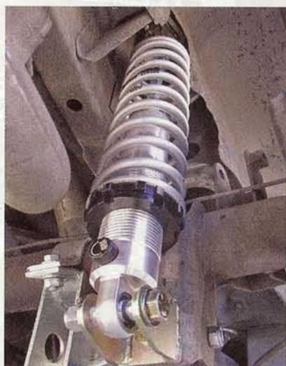
▲ Installation takes about one hour to complete. Using air and hand tools such as a 1/2-inch drive impact gun and 15/16-inch socket (for the shocks' upper mounting nut), a 3/8-inch drive ratchet, 3/4-inch socket, and a 3/4-inch wrench, setting UPR's Pro Series rear coilovers in the stock rear-shock location on a Fox or New Edge Mustang is easy.
