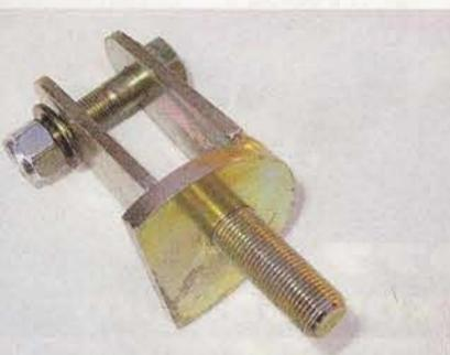
▲ Zinc-plated, lower (left) and upper shock mounts are secured on a 'Stang's rearend housing and up inside the rear shock towers. The fully welded brackets actually are stout and help prevent the springs from binding under hard side loads when cornering and under hard launches.
