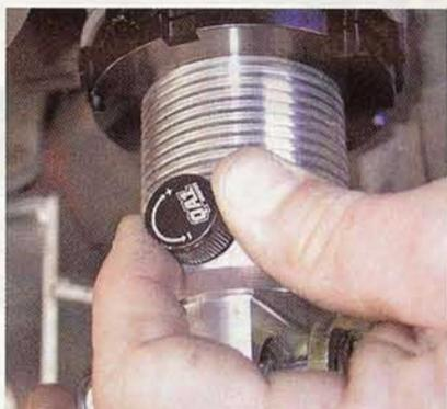
▲ Shock compression and rebound is calibrated by turning a single knob on each shock. The QA1s feature 12 settings, ranging from super-soft to ultra firm. For general street use, starting at the loosest setting, Greg rotates the knob clockwise (in the direction of the "+" symbol) until reaching the "third click" of firmness.
