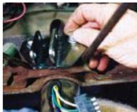
A bracket is then bolted to the couplers and will serve to anchor the support brackets for the pedal assembly.
