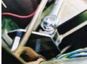
Todd then crawled back under the dash to bolt the support brackets to the dash mount plate.
