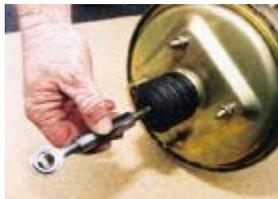
The power booster has a threaded, adjustable pushrod setup that needs to be assembled before the booster is bolted to the firewall bracket.
