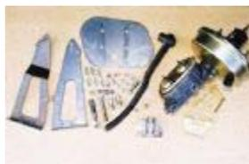
The complete kit comes with a new 8-inch booster, dual-chamber master cylinder, pedal arm, and all necessary brackets and hardware. Walton may make the bracket assembly available separately if there's enough interest.
