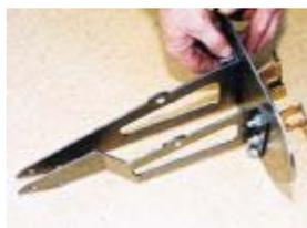
To make installation a one-man operation, Todd pre-assembled the brackets and firewall plate, leaving the bolts a little loose until it was all in the car.
