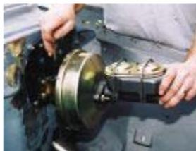
The master cylinder will still need to be removed and bench bled before the system is plumbed, bled, and put into service.
