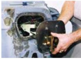
The bracket assembly was then slid in place through the firewall.
