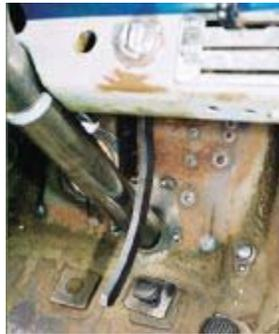
And that just about wraps things up! As you can see, the pedal arm hangs in a natural, comfortable position that's right in line with the original brake pedal. Walton plans to have a pedal pad designed for the kit by the time you read this.
