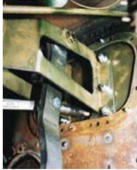
Back under the dash, the pedal arm can be bolted to its pivot (top) and secured to the pushrod.
