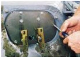
With the under-dash brackets bolted together, the firewall was secured using the supplied sheetmetal screws. All other hardware was cinched up at this time, too.
