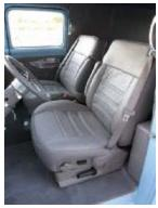
Louie at Mission Viejo Auto Interiors knocked the panel's leather upholstery out in record time. The front buckets are from a '00 <u>Chevy</u> pickup, and the overstuffed fold-down rear seat was snagged from a '00 Yukon.
