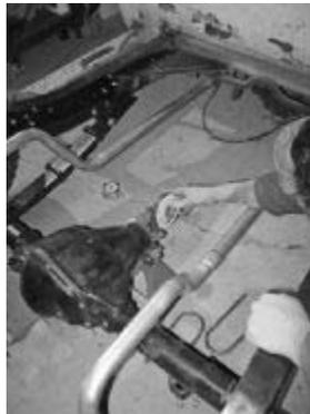
After careful removal of the old pads, the rearend was recentered between the framerrails, then the pinion angle set. Doing that revealed that even if the old pads would have worked, the pinion angle would have been way, way off, so it wasn't such a bad deal.
