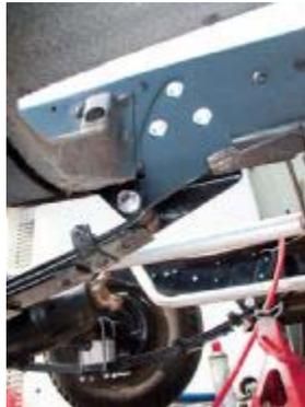
Start with the forward ends first (the side with the pre-installed bushing). A punch comes in handy to help guide the bushings into place.
