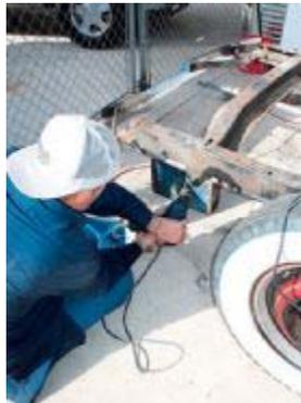
There was a great feeling of relief once the first spring hanger and its rivets were taken care of; unfortunately, there were still three more hangers and two shock brackets to remove! Once the last rivet is gotten rid of, run a 25/64 bit through each hole.
