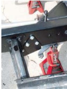
The forward spring hangers bolt directly to the existing holes in the frame, and are designed to fit without removal (let alone modification) of the stock E-brake cable brackets.
