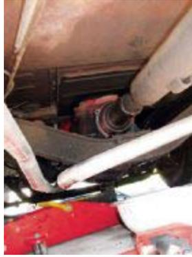
Since the springs were coming out with the rearend as one unit, the torque tube had to be disconnected from the tranny. First, all fluid was drained. Along with the threaded collar, there's also a plate mount that needs to come lose.
