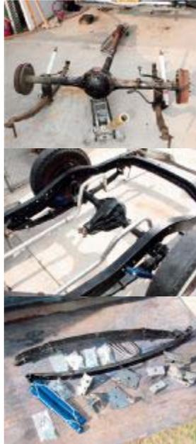
Whether or not you're losing the tube, if you want to lower your '47-54 Chevy 1/2-ton right, you gotta do it right with a parallel leaf kit from Walton Fabrication. Along with a set of beefy, modern-style springs, you also get U-bolts and five-hole plates, precision hangers and brackets, shocks, shock mounts, and all necessary hardware. Lowering blocks are also available for those wanting more of a drop, like me.
