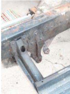
If you've never experienced the joy of removing beefy chassis rivets, you don't know what you're missing! The front and rear spring hangers as well as the shock mounts all attach to the frame with double-headed 3/8-inch rivets, each of which usually become very accustomed to being where they're at (in other words, stubborn to come out).
