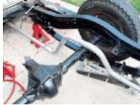
With the front and rear hangers attached with the supplied bolts and Nylocs, the new springs were ready to be installed.
