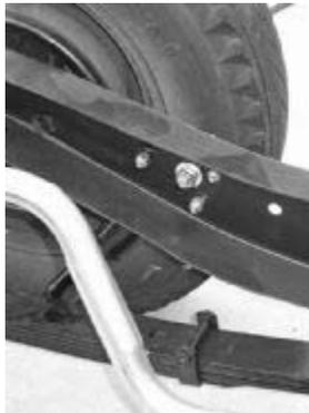
Walton provides reinforcing plates for the uppers, which bolt to the inside of the frame, with the studs on the opposite side, as shown.
