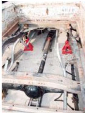
I've learned to be resourceful when doing jobs by myself. To remove the rearend assembly from beneath the truck without breaking an already broken back, I positioned the torque tube yoke on an old skateboard while walking the axle out with a floor jack.
