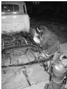
Anytime you weld on a rearend housing, chances of warping are very high, if not guaranteed (so be prepared to have it straightened professionally). With my 110V HTP, Jobe was able to turn the heat way down and still attain good-penetrating welds (in short sequences).
