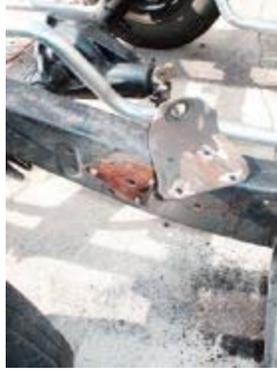
From there, a 4-inch grinder with a mean composite disc was used to rid what remained of the rivet heads. As you can see, there was still plenty of rivet left still to be removed.
