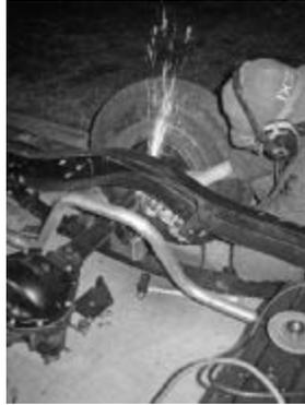
Once the leafs were hung, it became apparent that the old spring pads weren't going to fly--the Walton kit moves the springs inward a little over a half inch each side (it's really designed for a "stock" leaf-over setup to begin with). Considering my welding skills (or lack thereof), I made a 911 call to Jobe Jimenez to help with the additional chores. First off, the stock-but-flipped pads were cut off.
