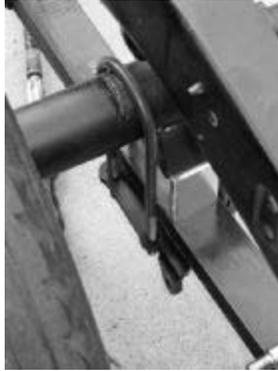
The following morning, I repainted the affected areas, then slid my lowering blocks between the springs and the housing. With the compressor ready and willing, I grabbed my 1/2-inch air ratchet and snugged the five-hole plates in place with the lower shock mounts on the outside.
