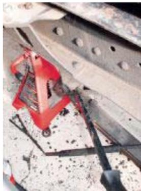
Unlike newer spring bushings, the early Chevy springs use threaded ends that you manually lube through zerk fittings. Buzz the bushings out, then, after making sure there's no load on the spring, pry the end out of the hanger.
