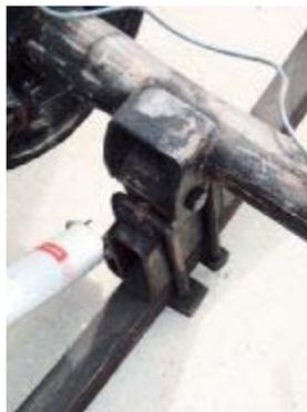
One of the reasons why the ride wasn't so favorable--5-inch blocks fab'd from steel tube. The KYB Gasadjust shocks were installed after acquiring, but actually worsened the ride by stiffening things up.
