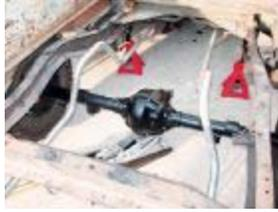
Rolled beneath the chassis, the Dana's overall width was right on the money, as expected. Now, it was simply a matter of removing the old suspension brackets and installing the Walton pieces.
