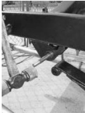
With the leaf spring still supported on the jack, the rear bushings can be installed, as shown. Using a bit of lubricated persuasion helps get the bushings in place without too much muscled effort.
