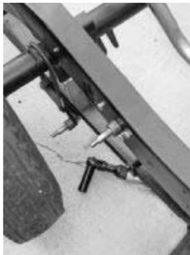
The shock studs were then bolted to the plates, followed by the uppers being installed on the framerrails.
