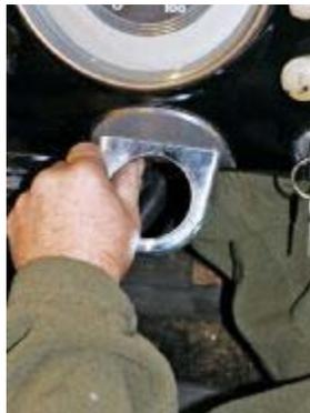
Once the stock column and steering box had been removed, the new column mount was attached to the dash using this plate to replace the stock '49 version.
