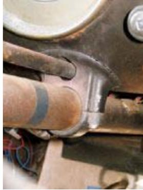
It's a different car, we know (the guys had already removed the stock column before we arrived at Walton), but here's a stock '49 column and its mount, which incorporates a hole for the column shift rod to pass through. The kit includes a replacement mount.
