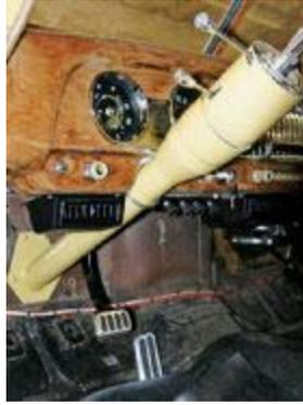
In '51-54 models, the new column can be installed with a simple U-bolt at the dash, as with this body color-painted column in a '53 woodie.
