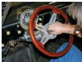
The dash mount bolts are tightened before the steering wheel is fitted. It will be clocked at alignment time.
