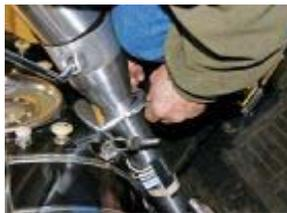
With the mount in place, it was simply a matter of feeding the lower end of the column through the stock hole in the firewall and installing the Allen bolts. Don't tighten 'em all the way just yet, though.
