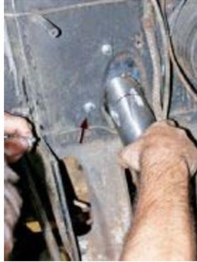
The holes in the plate lined up with the stock firewall holes (arrow), making locating and securing the firewall plate a snap.
