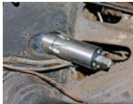
Here's the lower section of the column coming through the firewall. Again, you can see the tack-welded plate.
