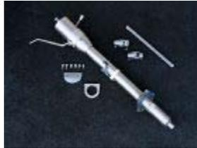
Here's the complete kit available from Walton Fabrication. The firewall-mount plate is tack welded to the column on this prototype but will be finish welded on production versions.
