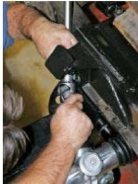
This particular '49 Chevy had already had Walton Fabrication engine mounts installed, along with a Total Cost Involved IFS and steering rack. The new universal joints supplied in the kit were installed on the rack and the column before the double-D shaft was installed and secured.
