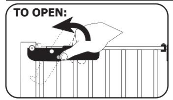
Push red safety button and lift landle  $90^{\rm o}$  upwards. Pull gate to open.
