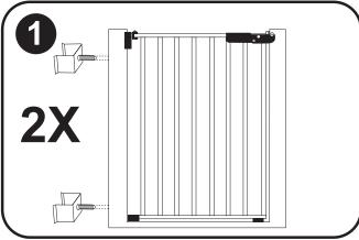
1. Choose appropriate screw-in clamps for your door. Screw clamps (A) into gate. These clips will fasten to open sliding door.
