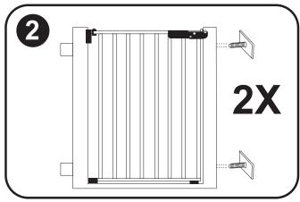
**2.** Screw stabilizer pads **(B)** into opposite side of gate. These pads will fit into C-channel of door frame.
