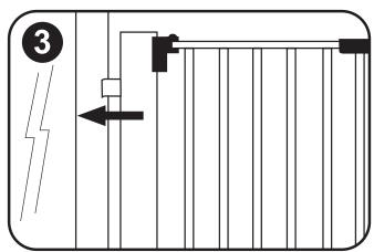
**3.** Attach gate to open door with clamps, fitting gate into door jam. Close door to lock in gate.
