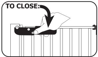
Close gate and lower lever back to original postion. Gate will click when locked.
