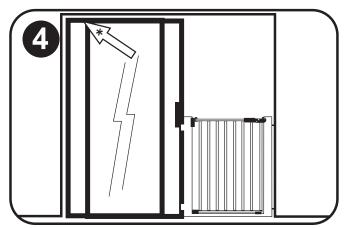
**4.** Screw door stop (**D**) to sliding track to secure sliding door (\*).
