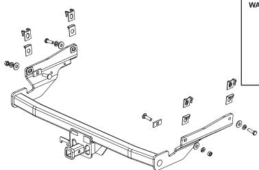
WARNING: ALTHOUGH THIS HITCH IS DESIGNED TO SAFELY TOW IT'S RATED LOAD, IT IS RECOMMENDED THAT YOU CONSULT YOUR VEHICLE OWNER'S MANUAL FOR FURTHER RECOMMENDATIONS OR LIMITATIONS. TRAILER BRAKES ARE RECOMMENDED FOR TOWING LOADS IN EXCESS OF 1500 lbs. BE SURE YOUR TRAILER HAS SAFETY CHAINS AND THAT EACH CHAIN WILL HOLD THE TRAILERS MAXIMUM GROSS WEIGHT.
