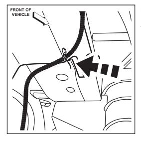
IF EQUIPPED, RE-INSTALL THE AUTO HEADLIGHTS WIRE HARNESS ON THE DRIVERS SIDE AND TRANS VENT TUBE ON THE PASSENGER SIDE WITH ZIP TIES
