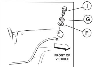
9 INSTALL REAR BOLT AND PLATE ASSEMBLIES TO VEHICLE FRAME
