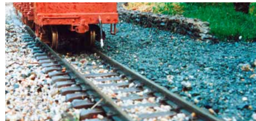
Code 332 rail is much taller than scale, and the bolts and brackets are European. However, this track is very robust and will take a lot of abuse. On the author's line, 90 percent of the track is code 332 and 10 percent is code 250.
