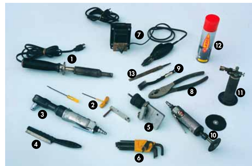
These are the basic tools for trackwork. 1. 175-watt soldering iron. 2. Allen wrenches with screwdriver handle and T-handle. 3. Air ratchet. 4. Atlas Super Saw. 5. Rail bender. 6. Allen wrench set. 7. Resistance soldering unit. 8. Pliers. 9. Stainless-steel wire brush. 10. Die grinder with extra cutting wheel. 11. Micro torch. 12. Butane gas.
