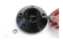
H. Adjust the collar at the bottom of the shock, up until it touches the upper cone for installation. We suggest adjusting the collar up to about 3 ½ inches from the top of the shock where the threads start down. This can be done after the top and bottom of the coilover is mounted to the car.
