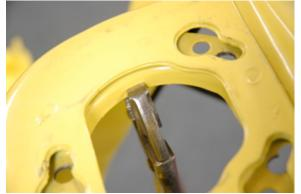
8. If you have ordered a negative roll system you will have an upper control arm template for drilling different locating holes. Note: If you did not order a negative roll system no template will be provided but you will have to drill the upper mounting holes out to 9/16
