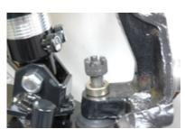
Install as shown and also install the upper ball joint through the spindle.
