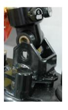
Tighten down the spindles to 80 foot pounds on the lower and 70 foot pounds on the upper.
