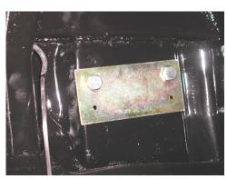
**diameter.** The original holes are ½ inch diameter. Slide a couple of ½ inch bolts through the template and inner shock tower. Position the new holes so they are below the original, center punch the holes.
